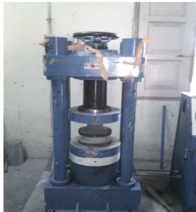
Fig 4.1 Test Set up for Compressive Strength Test
