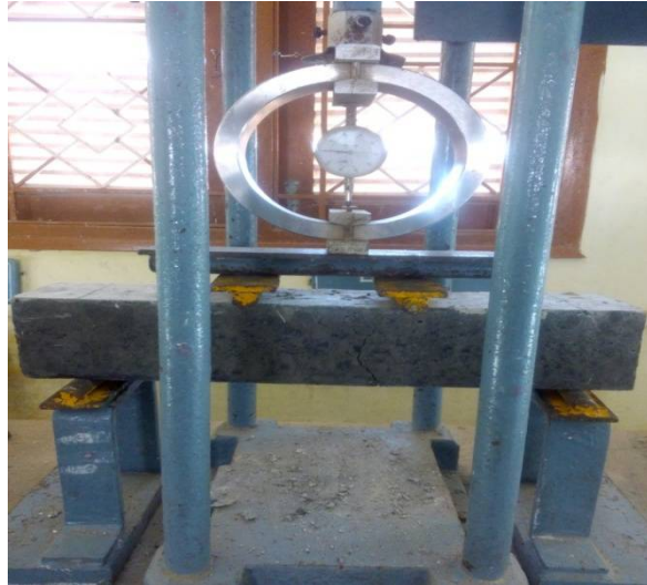
Fig 4.2 Test Set Up for Flexural Strength
